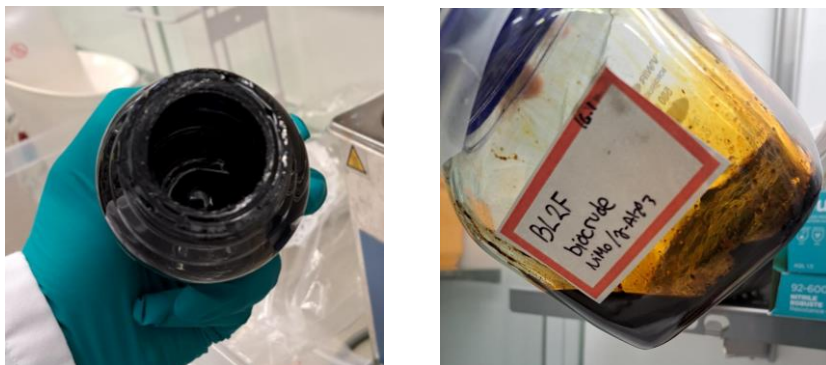
Figure 2. Biocrude before and after the hydrotreatment.
